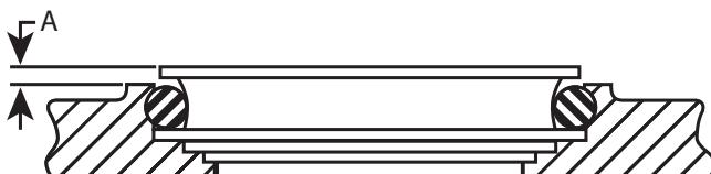
The difference in height around the ring must not be more than 1.0 mm. If small adjustments are necessary, do not push or pull directly on the seal ring. Use the installation tool to push down and your fingers to pull up uniformly on the rubber toric and seal ring.
