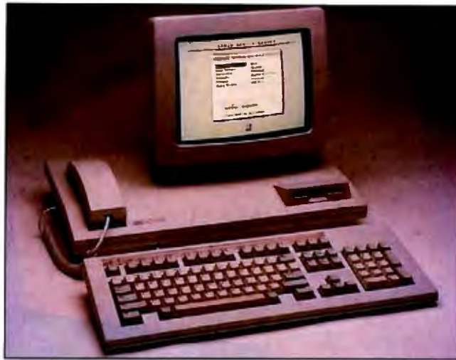
The Kowin Three uses a 68020 and dual 68000s.
