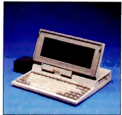
Photo A: The Toshiba T1000 is a 6½-pound 80C88-based laptop that operates from rechargeable batteries.
