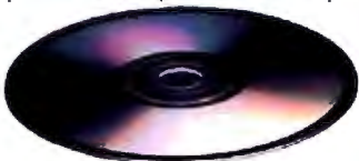
On a digital record, sound is carried by pits and spaces, which are read by a laser beam.
