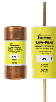
Figure 41: Low-Peak Class J fuses achieve rejection by their unique physical size that is unlike other CSA class fuses.
