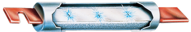
Figure 6: When subjected to a fault current, several sections of the fuse link melt almost instantly.
