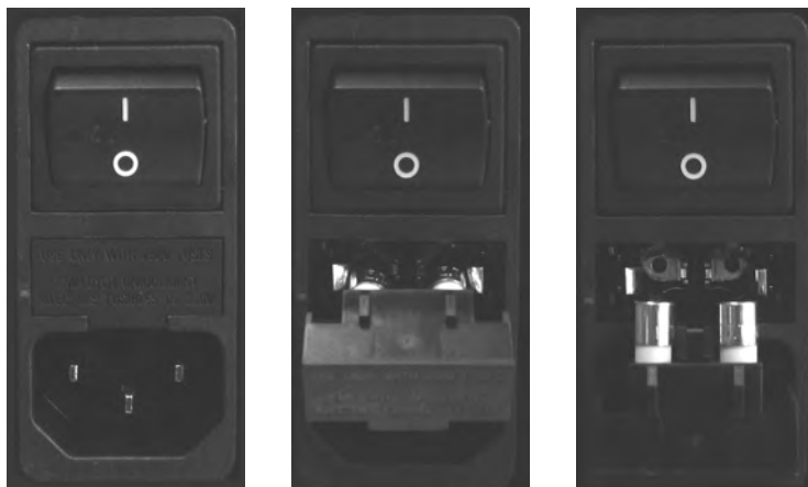
Figure 6. Replacing the fuse.
