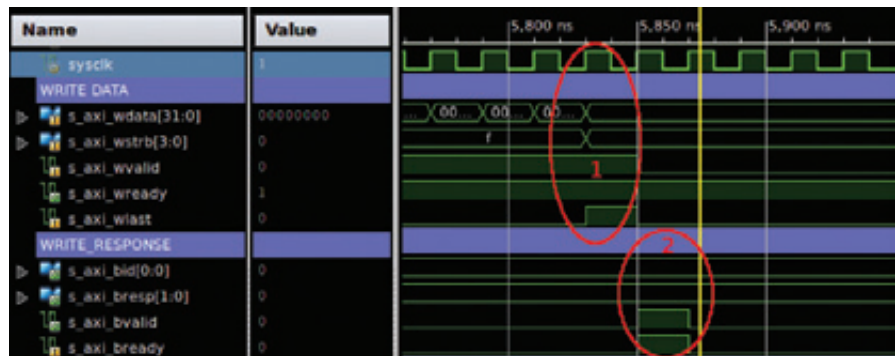
Figure 5 – The master labels the last word in the burst through the assertion of s_axi_wlast (1, top circle in screen shot). The slave informs the master whether the burst was successful through the write-response channel (2, bottom circle).
