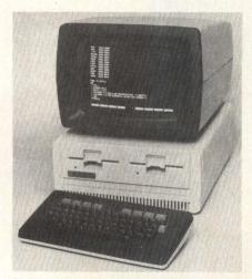
Realtime computer system. Desktop HP 1000 model 5, from Hewlett-Packard Co, includes HP 1000 L-series microcomputer, dual-disc drives, CRT, and keyboard
