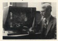
System uses simple rules to automatically combine elementary geometric solids such as cones, cylinders, and spheres to design solid mechanical parts. GMSOLID software is being developed by Dr John W. Boyse of General Motors Corp Research Laboratories in Warren, Michigan, and a team of engineers from the manufacturing and engineering staff.
