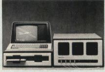
A desktop analyzer designed to meet demands of sophisticated requirements, the MicroModal<sup>TM</sup> was developed by GenRad, Vibration Analysis Div, 2855 Bowers Ave, Santa Clara, CA 95051, as a moderately priced microcomputer based analyzer for use in computer aided design and engineering. The system provides high speed animation on a 12" (30-cm) screen and stores 1M bytes of data on flexible media. Software is written in question and answer format for easy use.
