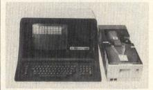
Series 550 consists of 16-bit minicomputer, 64k bytes of memory, disc controller capable of driving CDC 9455 Lark module drives, printer controller (parallel or serial), and a second asynchronous port for an additional CRT. 550-ns CPU has Data General compatible instruction set, and an adapter is available on the CPU board to accommodate security devices. System operates under IRIS, IOS, BITS, BLIS/COBOL, and MICOS operating systems. Bytronix Corp, 2701 E Chapman Ave, Fullerton, CA 92631.
