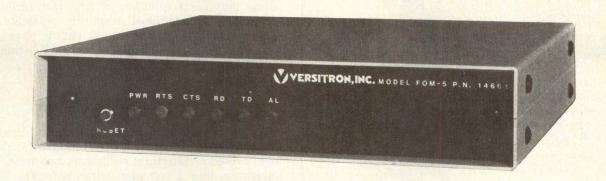
Fiber optic modems are ideally suited for many local data distribution applications since they offer several inherent advantages over conventional hardwired systems. These include immunity from rf and magnetic signals, increased bandwidth, and a significant improvement in the security of the data link.
