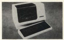
ID-100, a low cost serial communicating, ASCII terminal, is able to portray 8-color, character and symbol graphic images. The video color character graphics terminal, offered by ID Systems Corp, PO Box 393, Dublin, OH 43017, can function as a high performance 80- or 132-character/line replacement for the DEC VT-100.
