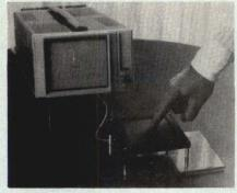
TouchGraphic operates using microproximity, high speed solid state sensing technology on both X and Y axes. Developed by TASA, Inc, 2346 Walsh Ave, Santa Clara, CA 95051, the unit can be used to replace trackball assemblies, as well as joysticks, lightpens, and field plotters.
