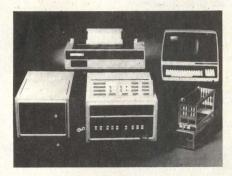
Bit slice development system. Advanced Micro Devices' AmSYS 29/10 features integrated logic analyzer and reduces debug time by emulating critical parts of target system
