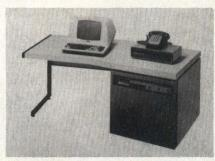
Supporting remote job entry, electrostatic plotting/printing, and graphics manipulation, the 444 remote plotting workstation accepts unsorted vectors as well as sorted vector, compressed raster, raster, and print data formats. Emulating HASP multileave remote workstations, the system, developed by Versatec, 2805 Bowers Ave, Santa Clara, CA 95051, provides IBM software and system protocol compatibility without requiring modification of the operating system.
