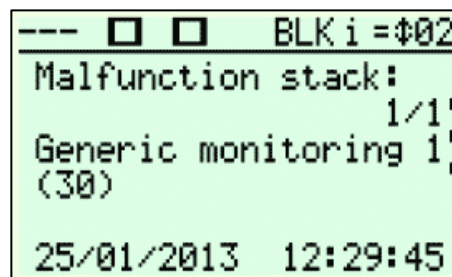
Figure 69: Representation of an entry in the stack memory with lock.
