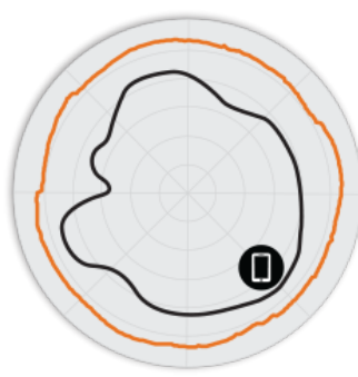
Figure 3. R730 5GHz Azimuth Antenna Patterns
