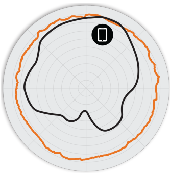
Figure 2. R730 2.4GHz Azimuth Antenna Patterns
