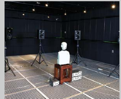
Measurement of acoustic characteristics using dummy heads in an anechoic room Researchers at Yamaha's Center for Advanced Sound Technologies are scientifically examining sound in its totality, including music, words, and noise. Research themes conducted in parallel include the emotional or healing impact of music and sound diffusion analysis. This work seeks to tap into the unknown potential that sound can derive.
