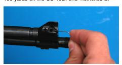
100 yards on the SU-16C and SU-16CA. Clockwise (in) moves the point of impact up and counter-clockwise (out) moves it down.
