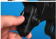
It will snap onto the forend with a lot of force. To unfold the stock, simply pull down to unsnap the stock and extend it to lock.
