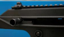
correctly with the screw head on the inside of the receiver. The rear of the dustcover should be flush with the back of the bolt carrier. Align the operating handle hole in the carrier with the cut-out in the receiver and insert the operating handle. Push the carrier up slightly so that the operating handle aligns with the slot for it and the recoil spring tube is parallel with the barrel of the rifle.
