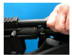
inspect the chamber to make sure it is empty. Pull back on the operating handle to release the bolt stop and release the operating handle to close the chamber. Push the remaining cartridges in the magazine forward and out.
