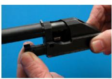
not be inserted correctly. Insert the firing pin pin into the bolt carrier from the left side. DO NOT FORCE THE FIRING PIN PIN. If it does not go in easily, check that the firing pin is installed correctly. Check the operation of the bolt and firing pin to be sure that they move freely.
