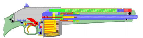
receiver has an aluminum insert molded into the front to accept the barrel and the serial number.
