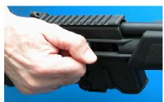
the last round has been fired. The SU-16 has an automatic bolt stop so after the last round is fired the bolt will lock open. Remove the empty magazine by pressing the magazine catch located on the right side of the receiver and pull out the empty magazine. To continue shooting, simply insert a full magazine into the magazine well, firmly push it up until it locks, and pull back and release the operating handle to release the bolt stop and feed the next round. The rifle is now ready to fire.
