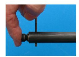
CAUTION: The piston head is under pressure from the compressed recoil spring and the piston head and recoil spring can easily fly out and injure yourself or bystanders, always keep a hand on the piston head and point the piston head in a safe direction when removing it.
