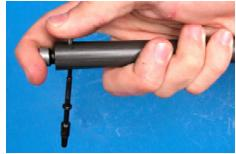
towards the top of the bolt carrier. Check the operation of the recoil spring by lightly pulling on the recoil spring tube to compress the spring.
