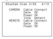
**CAMERA Cable**: Camera cable connection status **CAMERA Data**: Camera data transmission status **CAMERA Power**: Camera power supply status
