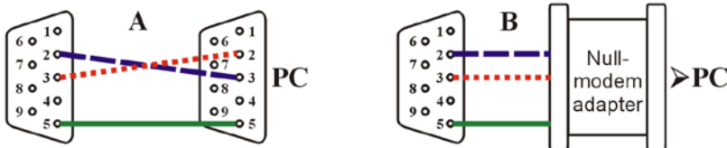
Figure 3: Connecting the RS-232 Port
