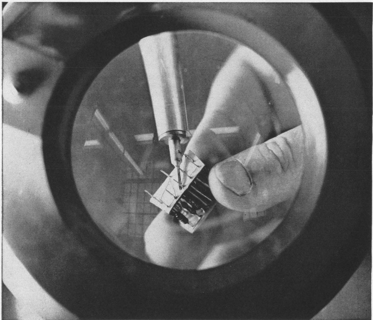
View through magnifier shows how joint in cordwood module is made by touching it to drop of solder on iron.
