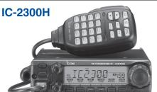
The IC-2300H 2 meter FM mobile has a large 4level backlit LCD that may be set to green, yellow or amber. The receiver covers 136-174 MHz and the transmitter delivers 65, 25, 10 or 5 watts. Improved receive IMD helps provide protection from strong signals such as pager signals. With: 207 alpha memories, 3-way priority watch and independently programmable Rx/Tx and tone squelch. There is an FM narrow mode. With HM-133V remote mic. 5.51 x 1.6 x 6.4 inches.
