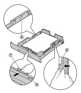
5 Insert the paper input tray into the unit, lifting the front part of the tray. Then push it completely into the unit.
