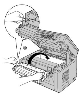
Make sure that the arrows (<sup>®</sup>) match, to install the drum and toner cartridge correctly.
