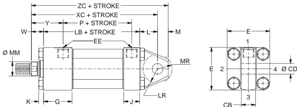
**BE Mount Single Rod End – Envelope and Mounting Dimensions**
