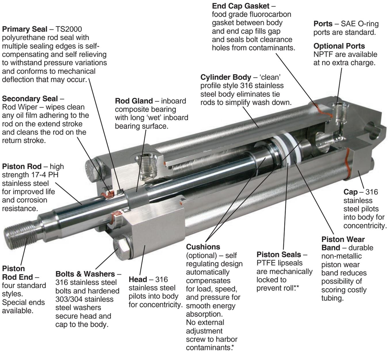
\* When cushions are specified on 1½", 2", 2½" bores with oversize rod, a fixed cushion without adjusting screw is supplied on the head end. Fixed cushion rate of deceleration is constant and does not vary with load, speed, and pressure like self-regulating style cushions.
