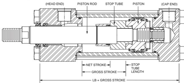
When specifying cylinders with long stroke and stop tube, be sure to call out the net stroke and the length of the stop tube. Machine design can be continued without delay by laying in a cylinder equivalent in length to the NET STROKE PLUS STOP TUBE LENGTH, which is referred to as GROSS STROKE.
