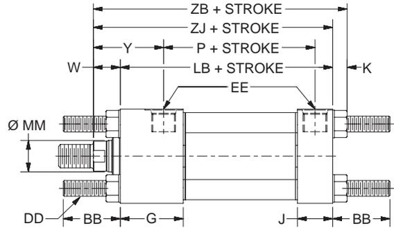
**T, TB, TC, TD Mount Single Rod End – Envelope and Mounting Dimensions**
