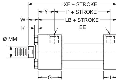
**HH Mount Single Rod End – Envelope and Mounting Dimensions**
