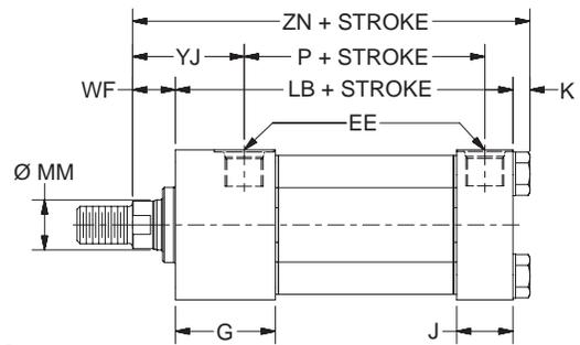
**JJ Mount Single Rod End – Envelope and Mounting Dimensions**
