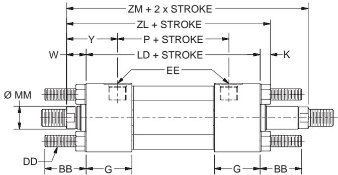
**T, TB, TD Mount Double Rod End – Envelope and Mounting Dimensions**
