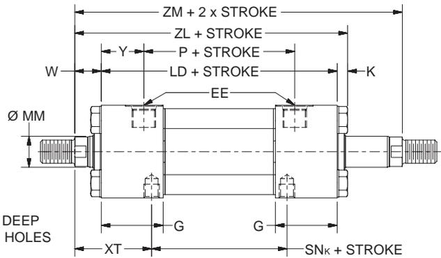
**F Mount Double Rod End – Envelope and Mounting Dimensions**
