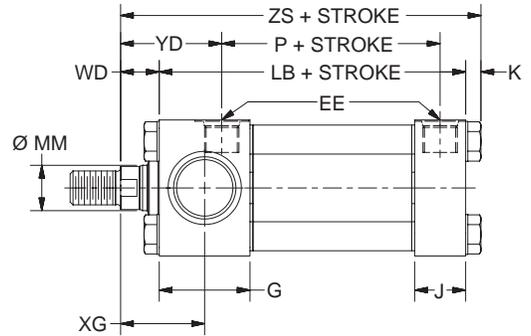
**D Mount Single Rod End – Envelope and Mounting Dimensions**
