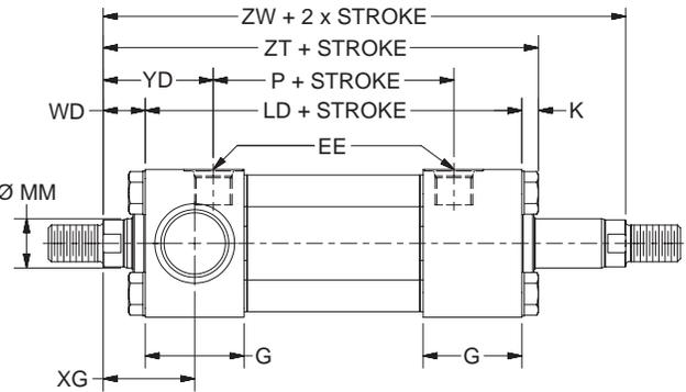
**D Mount Double Rod End – Envelope and Mounting Dimensions**
