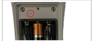
Figure 12: Alignment Access Hole Location
