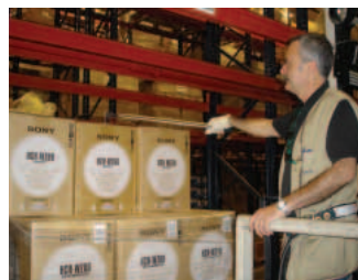
The Barcelona Distribution Center of Sony España, S.A., won the 2006 OHS Best Practice Award for developing this box-pulling tool, which prevents back strain in warehouse operations.
