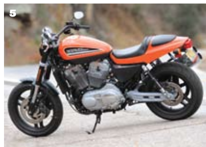
1) Inverted 43 mm Showa forks, lightweight aluminum wheels, and Nissin four-piston caliper brakes offer telepathic performance. 2) Dual upswept mufflers highlight the XR's heritage. 3) Form follows function with no-frills instrument cluster. 4) Active intake system, downdraft EFI, and 10.0:1 compression add muscle. 5) Rear-set footpegs and a 39-degree lean angle speak to your inner-Scott Parker.
