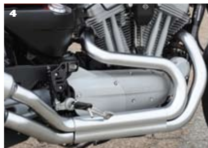
1) Inverted 43 mm Showa forks, lightweight aluminum wheels, and Nissin four-piston caliper brakes offer telepathic performance. 2) Dual upswept mufflers highlight the XR's heritage. 3) Form follows function with no-frills instrument cluster. 4) Active intake system, downdraft EFI, and 10.0:1 compression add muscle. 5) Rear-set footpegs and a 39-degree lean angle speak to your inner-Scott Parker.
