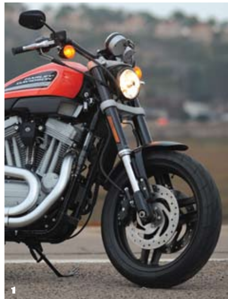
1) Inverted 43 mm Showa forks, lightweight aluminum wheels, and Nissin four-piston caliper brakes offer telepathic performance. 2) Dual upswept mufflers highlight the XR's heritage. 3) Form follows function with no-frills instrument cluster. 4) Active intake system, downdraft EFI, and 10.0:1 compression add muscle. 5) Rear-set footpegs and a 39-degree lean angle speak to your inner-Scott Parker.
