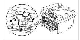
Put the drum unit and toner cartridge assembly back into the machine.
