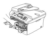
2 Clean the primary corona wire inside the drum unit by gently sliding the blue tab from right to left several times.
