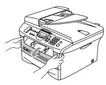
2 Pull out the drum unit and toner cartridge assembly.
