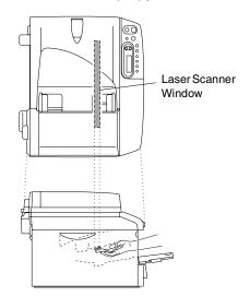
4 Put the drum unit and toner cartridge assembly back into the machine.
