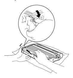
4 Put the toner cartridge back into the drum unit until you hear it lock into place. If you put it in properly, the lock lever will lift automatically.
