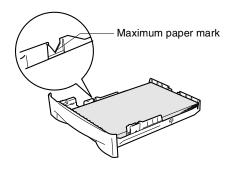
Dut the paper tray firmly back in the machine and unfold the output paper tray support flap before you use the machine.
