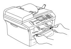
Using both hands put one sheet of paper in the manual feed slot until you feel the front edge of the paper touch the paper feed roller. Let go of the paper when you feel the machine feed the paper in a short distance.
