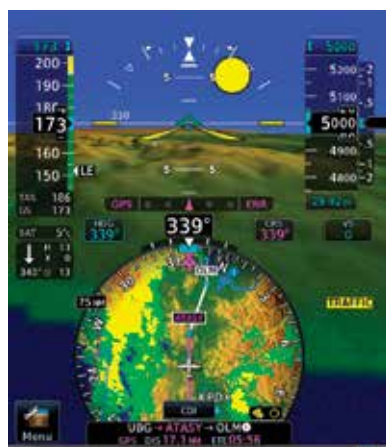
With Garmin SVT-capable flight displays, traffic can be depicted in a 3-D format. As targets get closer, the symbols get larger.
