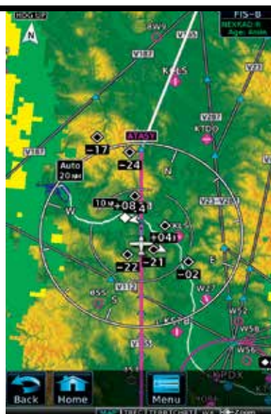
Integration of traffic and weather on a Garmin moving-map display provides critical situational awareness of potential flight-path conflicts.
