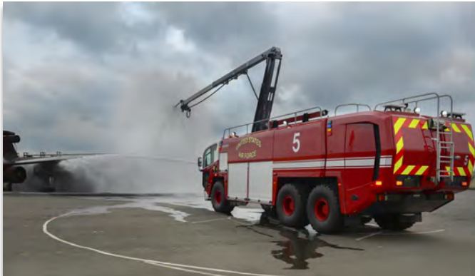
Airman 1st Class Thomas Smith, 373th Civil Engineer Squadron firetruck driver operator, demonstrates the Striker 3000 fire truck's capabilities at Yokota Air Base, Japan, June 28, 2016. The Striker 3000 is Yokota's newest firetruck, equipped with a boom that extends 75 feet longer than older models, giving it a total range of 750 feet. (U.S. Air Force photo by Airman 1st Class Baker/Released)
