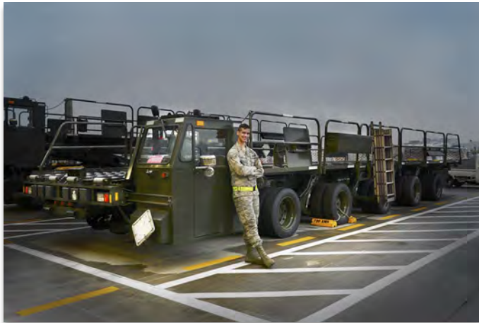
Airman 1st Class John Thomas Dennis, 730th Air Mobility Squadron air freight technician, poses for a photo with a 60k Tunner at Yokota Air Base, Japan, June 29, 2016. The 60k Tunner is the military's largest K-loader, vehicles used to on- and off-load aircraft cargo. (U.S. Air Force illustration by Airman 1st Class Baker/Released)
