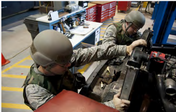
Senior Airman Thomas Harvey and Senior Airman Dillon Goulet, 51st Logistics Readiness Squadron mission generating and vehicle maintenance journeymen, remove a leaking radiator from a vehicle during Exercise Beverly Herd 16-2 on Osan Air Base, Republic of Korea, Aug. 25, 2016. Harvey and Goulet continue to enable base operations and defense of the base by fixing vehicles so they can be returned to the field. (U.S. Air Force photo by Staff Sgt. Jonathan Steffen)
