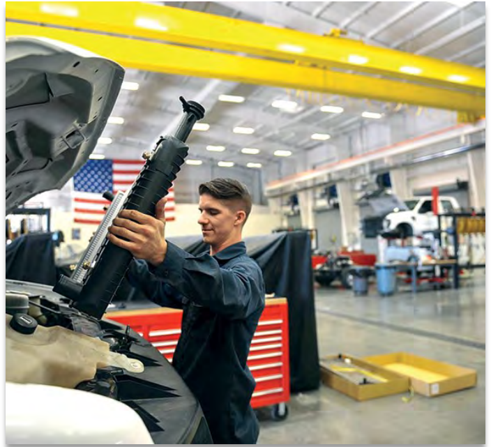
Senior Airman Levi Powers, 99th Logistics Readiness Squadron Vehicle Management Flight general purpose vehicle maintainer places a new radiator into a vehicle at Nellis Air Force Base, Nev., May 3. The flight is able to manage more than 1,500 vehicles, due to its 80,000 square foot state-of-the-art-facility.
