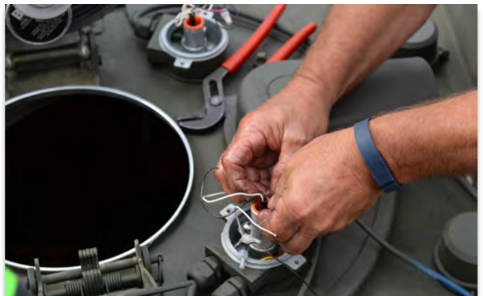
Joe Robinson, 4th Logistics Readiness Squadron fire truck and refueling maintenance technician, adjusts a fuel sensor on the new Isometrics R-11 Refueler, May 17, 2016, at Seymour Johnson Air Force Base, North Carolina. The new R-11 has more automatic features to help prevent fuel waste and accidents. (U.S. Air Force photo by Airman 1st Class Ashley Williamson)
