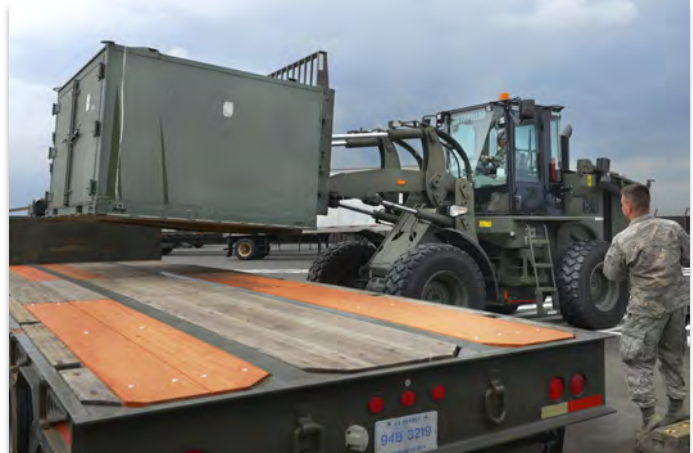
Airman Jalen Johnson 374th Logistics Readiness Squadron vehicle operator and dispatcher, uses a 10k all-terrain forklift to load cargo onto a trailer while spotted by Airman 1st Class Dube Johnson, 374 LRS vehicle operator and dispatcher, at Yokota Air Base, Japan, June 29, 2016. The 374 LRS uses 10ks, which can lift and transport up to 10,000 pounds, to support cargo operations throughout Yokota. (U.S. Air Force photo by Airman 1st Class Baker/Released)
