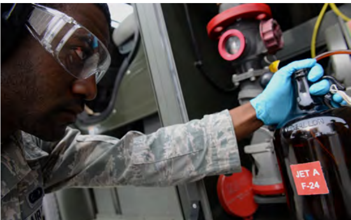
Senior Airman Terrence Baker, 4th Logistics Readiness Squadron petroleum, oil, and lubricants fuels lab technician, takes fuel samples from the new Isometrics R-11 Refueler, May 17, 2016, at Seymour Johnson Air Force Base, North Carolina. The R-11 has the ability to carry fuel to jets and pump fuel from underground hydrant systems to refuel aircraft. (U.S. Air Force photo by Airman 1st Class Ashley Williamson)
