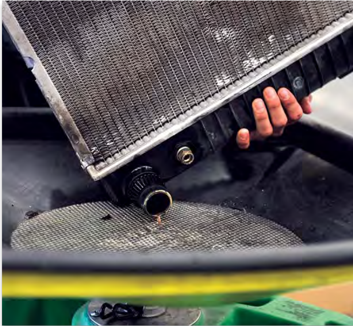
Senior Airman Levi Powers, 99th Logistics Readiness Squadron Vehicle Management Flight general purpose vehicle maintainer drains fluid from an old radiator at Nellis Air Force Base, Nev., May 3. Powers and many other members of the vehicle management flight maintain and manage the vehicle fleet at Nellis AFB.
