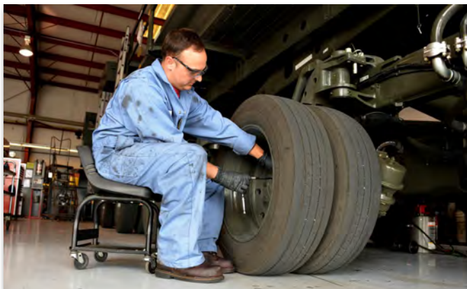
Cory Bellmore, 60th Logistics Readiness Squadron heavy vehicle mechanic, checks the level of the hubs on a Tunner 60K aircraft loader April 26, 2016, at Travis Air Force Base, California. Travis Air Force Base has a total of 17 Tunner 60K aircraft loaders supporting aerial port squadron operations, the largest 60K loader fleet in the Air Force. (U.S. Air Force photo by Staff Sgt. Charles Rivezzo)
