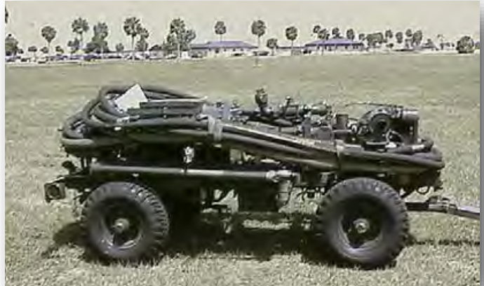
PMU-27: The PMU-27 is a trailer-mounted, engine-powered unit consisting of a 50-gpm pump, filter separator, meter, hoses, connections, and nozzles. It is designed to support servicing of small aircraft and transfer of small quantities of fuel.
