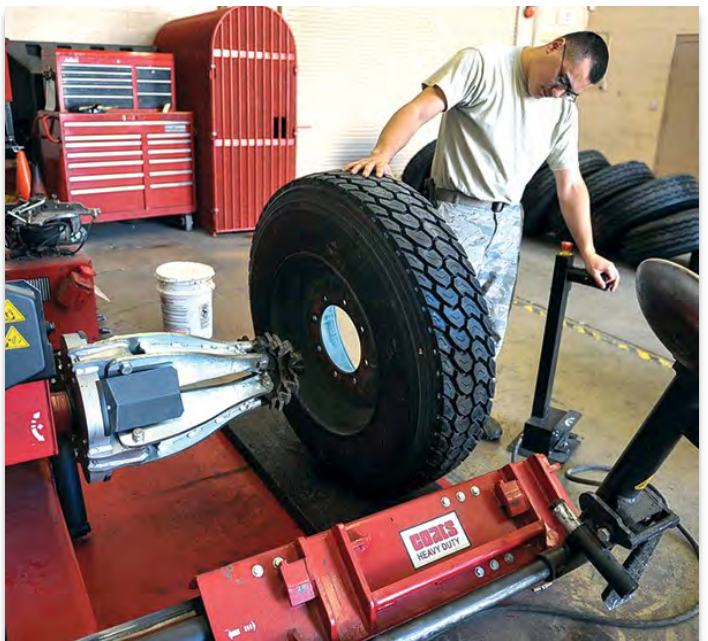
Staff Sgt. Joseph Petrie, 99th Logistics Readiness Squadron Vehicle Management Flight tire shop maintainer loads a tire onto a machine at Nellis Air Force Base, Nev., May 3. The machine allows Airmen in the shop to easily load and unload tires from vehicles.
