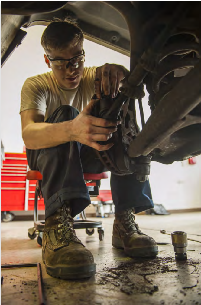
U.S. Air Force Airman 1st Class William Leonard, 18th Logistics Readiness Squadron vehicle mechanic, performs a ball joint replacement in the special vehicles shop April 14, 2016, at Kadena Air Base, Japan. The 18th LRS is the largest LRS in the Air Force and is composed of 757 authorized personnel. (U.S. Air Force photo by Airman 1st Class Nick Emerick)
