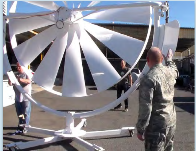
Natural Power Concepts personnel and Lt. Col. Scott Fitzner, of the AFRL Materials and Manufacturing Directorate, inspect the spoke wheel medium wind power system, one of a number of energy-harvesting technologies being installed as part of the five-year, $20 million cooperative agreement with AFRL that will establish a microgrid demonstration project at Joint Base Pearl Harbor-Hickam in Hawaii. (Courtesy photo/Hawaii Center for Advanced Transportation Technologies)
