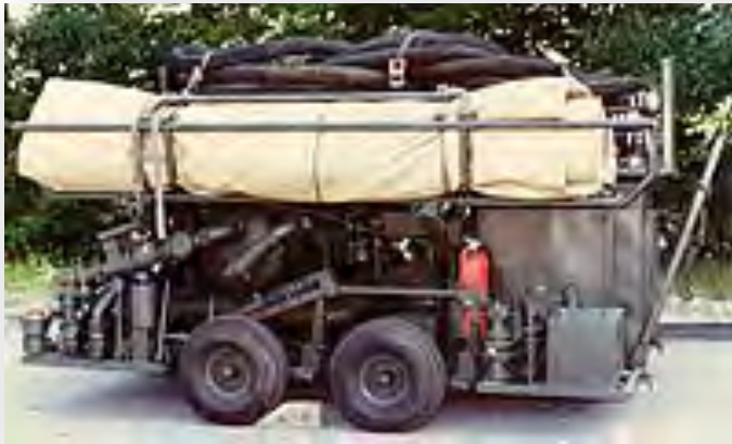
R-14: By far, the most widely used and one of the most versatile systems is the R-14. The R-14 is a portable, hydrant-refueling system that can be airlifted or ground shipped anywhere in the world and made fully operational in a matter of hours.
