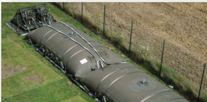
ABFDS: The ABFDS is an aerial, fuel-delivery system that enables aircraft to rapidly transport fuel to locations close to or behind enemy lines. It consists of two 3,000-gallon aerial bladder tanks, two pumping modules, a meter, and hoses.
