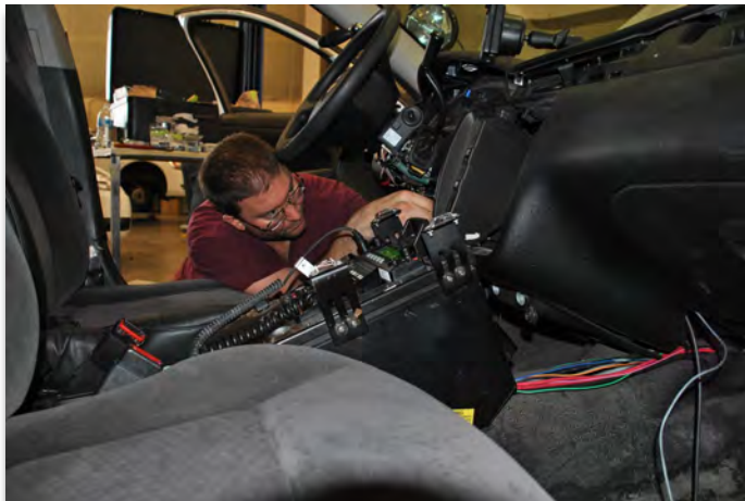
A mechanic with the 502nd Logistics Readiness Squadron at Joint Base San Antonio-Fort Sam Houston installs one of the idle-reduction systems being tested on security forces vehicles. (U.S. Air Force photo by Carole Chiles Fuller)
