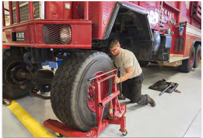
Airman 1st Class Thomas Zak, 96th Logistics Readiness Squadron, pushes a 5,000-pound serviceable axle and differential assembly under Tanker 46 Nov. 10 at Eglin Air Force Base, Fla. The part was procured from a Tyndall AFB fire truck slated for the salvage yard and re-installed into Tanker 46, a broken 1989 model 2,000-gallon water tanker fire truck. The repair job saved the Wing $25 thousand and maintained response readiness. (U.S. Air Force photo/Ilka Cole)
