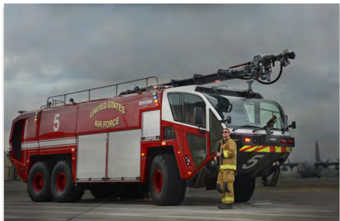
Airman 1st Class Thomas Smith, 374th Civil Engineer Squadron firetruck driver operator, poses for a photo with a Striker 3,000 fire truck at Yokota Air Base, Japan, June 28, 2016. The Striker 3000 is Yokota's newest fire truck and is specialized with features like the hull-piercing snozzle to combat aircraft-related fires. (U.S. Air Force illustration by Airman 1st Class Baker/Released)
