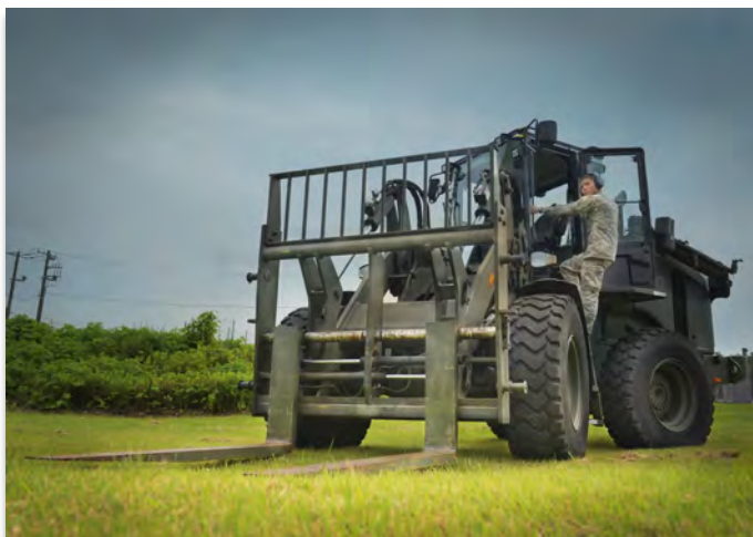
Airman Jalen Johnson 374th Logistics Readiness Squadron vehicle operator and dispatcher, poses for a photo with a 10k all-terrain forklift at Yokota Air Base, Japan, June 29, 2016. The 10k is essential to Yokota operations for its ability to lift, load and transport heavy cargo such as aircraft-part pallets. (U.S. Air Force illustration by Airman 1st Class Baker/Released)
