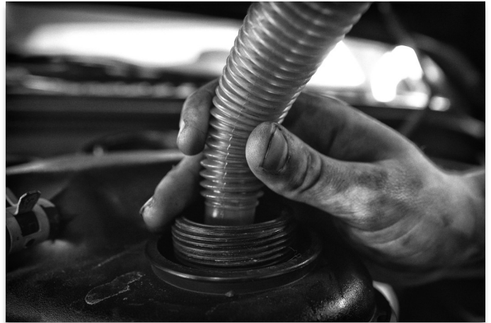
U.S. Air Force Senior Airman Michael Siters, 374th Logistics Readiness Squadron vehicle maintenance journeyman, funnels antifreeze into a government vehicle at Yokota Air Base, Japan, April 13, 2016. The shop ensures the upkeep of all Yokota's government vehicles by providing regular maintenance and repair. (U.S. Air Force photo by Senior Airman Delano Scott/Released)
