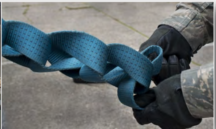
RAMSTEIN AIR BASE, Germany -- Airman 1st Class Brody Ellyson, 86th Vehicle Readiness Squadron vehicle operator, ties a loading strap using a daisy-chain technique Aug. 19, 2016 at Ramstein Air Base, Germany. Once the cargo is ready to be unloaded, the daisy-chain technique enables the strap to be undone with one pull. (U.S. Air Force photo/Senior Airman Tryphena Mayhugh)
