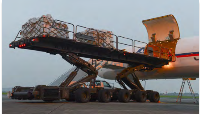
Airmen load cargo pallets from a Boeing 757 onto a 60k Tunner at Yokota Air Base, Japan, June 29, 2016. The 60k Tunner can hold up to 60,000 pounds of cargo and elevates up to 222 inches. (U.S. Air Force photo by Airman 1st Class Baker/Released)
