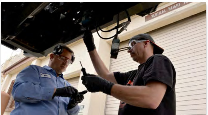
Sean O'Leary, left, and Michael Dickie, right, both from the 60th Logistics Readiness Squadron install a limit switch on an aircraft cargo loader April 26, 2016, at Travis Air Force Base, California. (U.S. Air Force photo by Staff Sgt. Charles Rivezzo)
