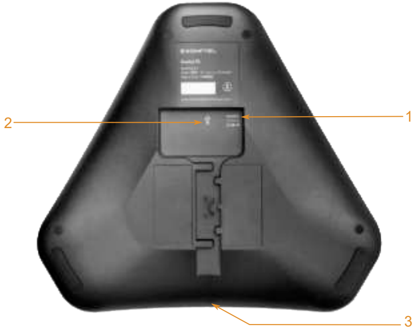
Figure 2: Connection layout of Konftel 70
