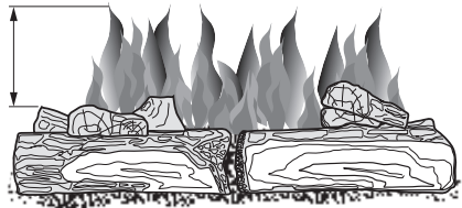
Figure 27 - Incorrect Burner Flame Pattern
