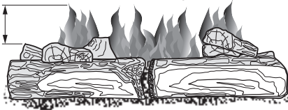
Figure 26 - Correct Burner Flame Pattern
