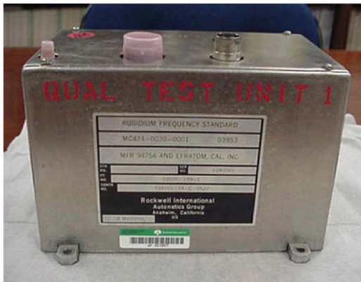
Qualification Model of the first GPS atomic clock, built by Rockwell International working directly with Efratom, a small German company.
