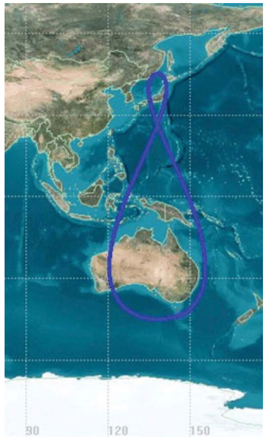
Figure 6. The Japanese QZSS has a similar constellation to an early proposal for GPS under 621B.
