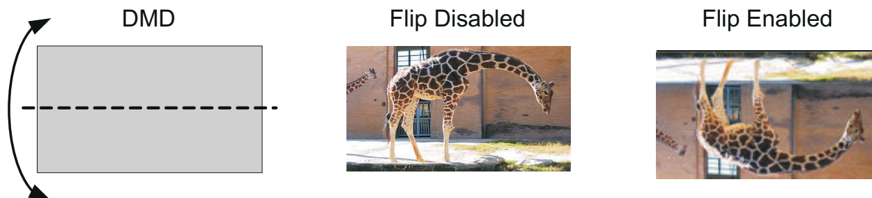
Figure 2-2. Image Short-Axis Flip Example
