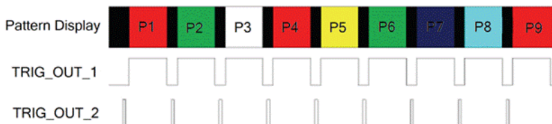
Figure 2-9. Pre-Stored Pattern Mode Timing Diagram Example
