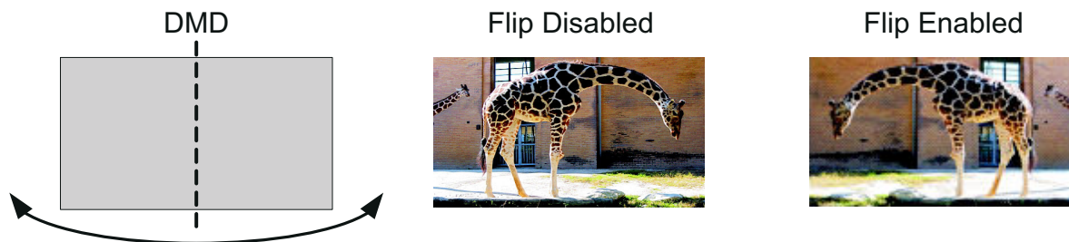
Figure 2-1. Image Long-Axis Flip Example
