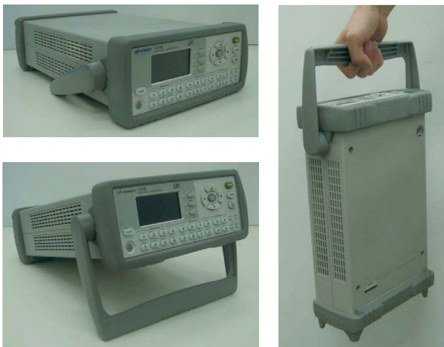
Figure 2-1 Handle positioning for bench operation
