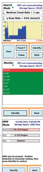
**GAMMA DOSE RATE**: Gamma Dose Rate is monitored by the HPGe detector and by an internal compensated GM tube. The dose rate is displayed at all times. Dose rate units may be chosen as  $\mu Sv/hr$  or mrem/hr.
