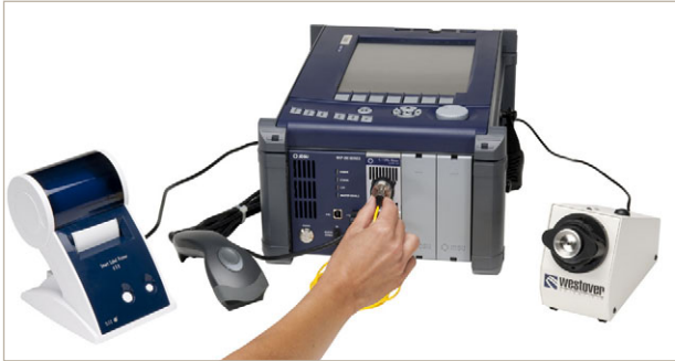
Figure 8: Example using the JDSU FVD to verify the connector end face of the jumper under test
