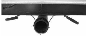
Black/Grey Tank Drain and Valves
