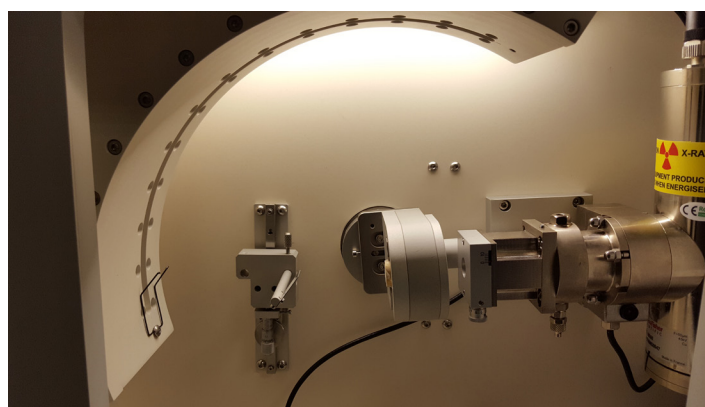
Figure 2: ARL EQUINOX 100 in transmission measurement mode
