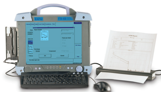
■ The FTB-400 with print function and external printer.
