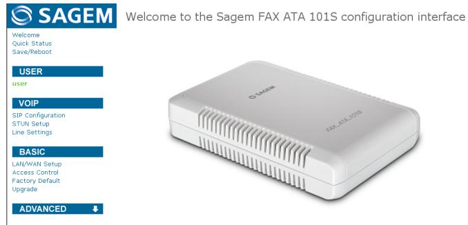
You can then assign an IP address (fixed or dynamic via a DHCP server) to the Sagem Fax ATA 101S WAN port via the Web setup interface.
