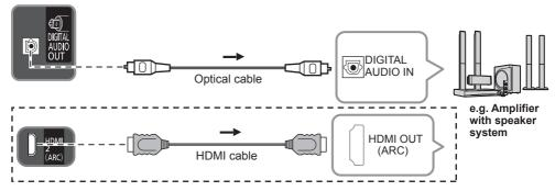
HDMI connection is available if connected audio equipment has ARC (Audio Return Channel) function. Select ARC output HDMI 2/HDMI 4 according to connected device.
