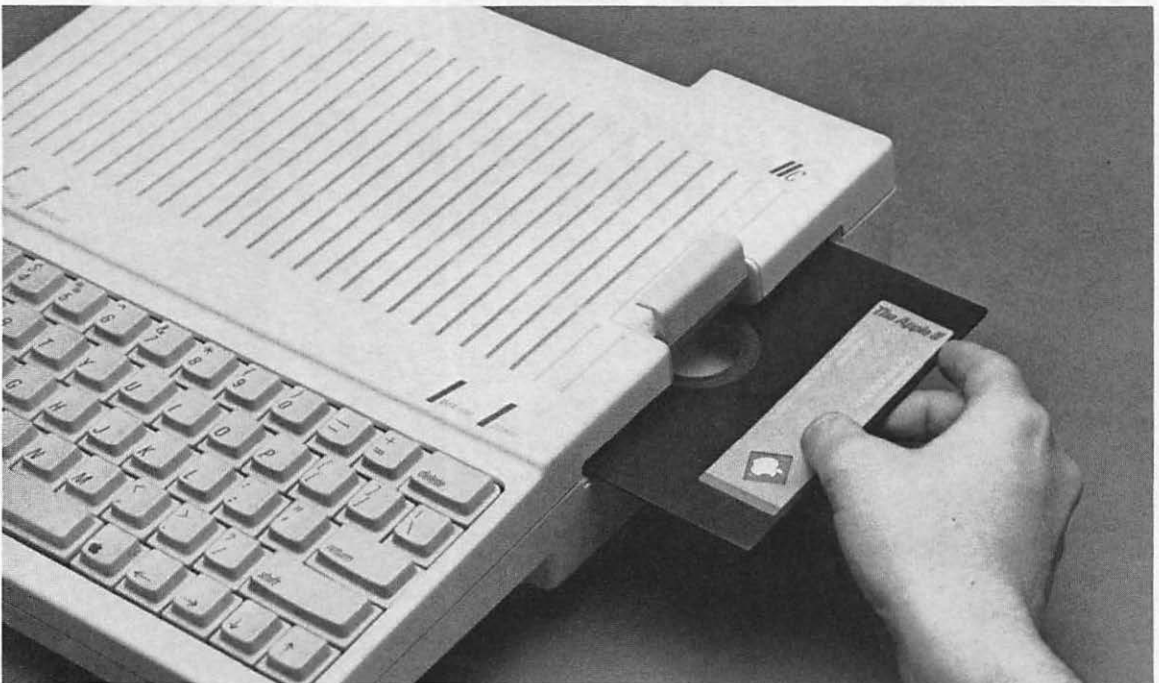
Fig. 2-5. The Apple IIc has a built-in, single-sided disk drive (courtesy of Apple Computer, Inc.).
