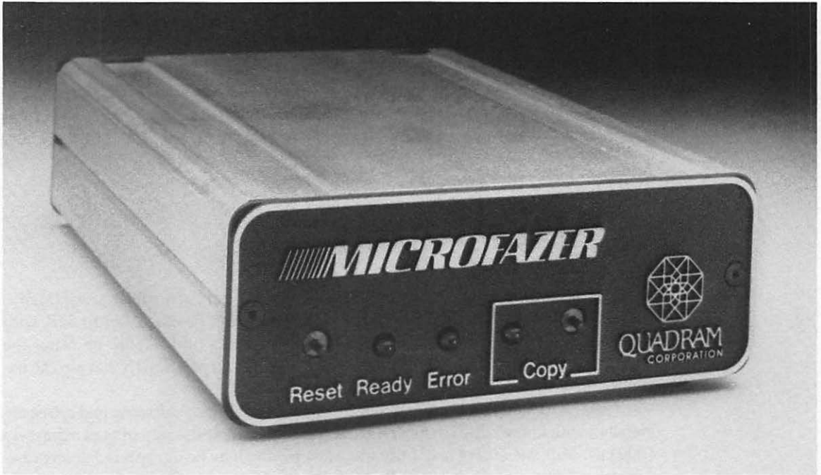
Fig. 20-5. The Microfazer buffer is available in several memory configurations, including 256K and 512K (courtesy of Quadram Corporation).
