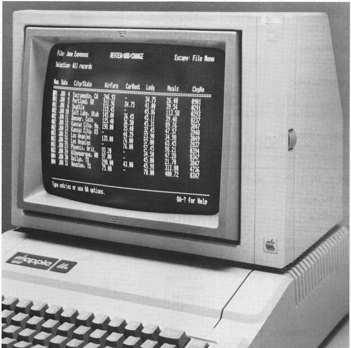
Fig. 9-2. The Monitor IIe will work with all the members of the Apple II family (courtesy of Apple Computer, Inc.).
