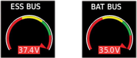
Essential Bus and Battery Over Voltage
