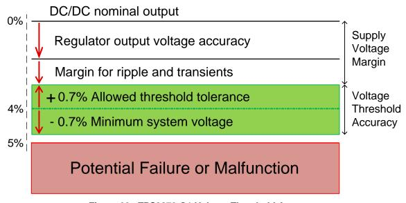
Figure 20. TPS3870-Q1 Voltage Threshold Accuracy
