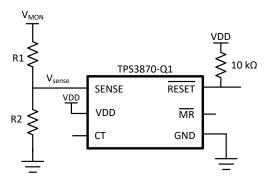
Figure 23. Adjustable Voltage Threshold with External Resistor Dividers
