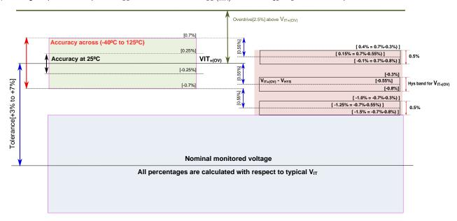
Figure 1. Voltage Threshold and Hysteresis Accuracy
