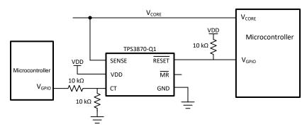
Figure 25. Window Voltage Monitoring with RESET Latch
