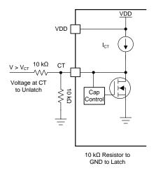
Figure 22. RESET Latch Circuit
