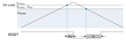
Figure 18. RESET output
