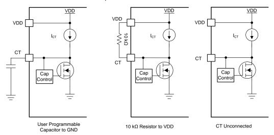
Figure 21. CT Charging Circuit
