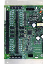
Panel 1 Set Configuration (Modbus Register 6) to Top Feed (0)
