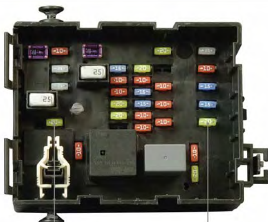
F102 20 Amp Yellow – Cigar Lighter Instrument Panel & Power Outlet Left Rear Cargo Area
