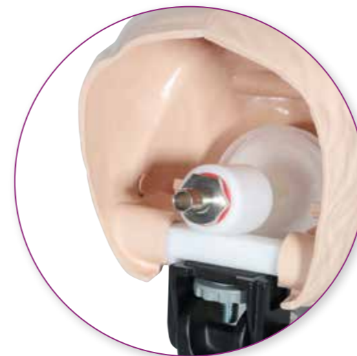
Filter Holder and Adapter located in a cavity behind the face model's lips
