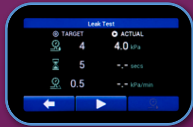
Leak test screen
