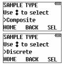
To select COMPOSITE or DISCRETE sampling use up or down arrow and push SEL(F3).
