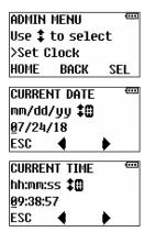
Press the number buttons to type the current date and hours (using 24-hour format). Press ENTER to accept the date and move to time. When finished the screen will advance to ADJUST LCD screen.
