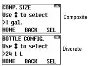
When the bottle and sample size is programmed the control will automatically set the max bottle limit to 90%.
