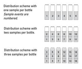
This SAMPLES PER BOTTLE feature can be combined with the BOTTLES PER SAMPLE EVENT (Section 3.5.4) to build more complex distribution schemes, sometimes known as
