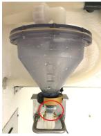
Figure 5-3 Location of the chamber discharge fitting
