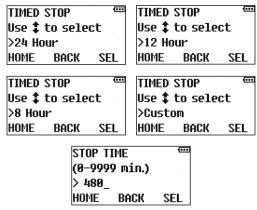
This feature is useful for applications that require the collection of a total sample volume proportional to the flow volume over a specific duration. An example of this would be a flow-weighted composite sample representative of the total daily flow volume (24 hours). If the application does not limit the sample collection to a specific duration, enter none.
