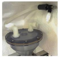
Figure 5-4 Connecting the vacuum/pressure tubing
