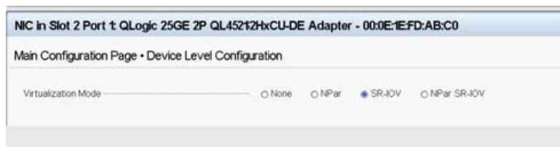
Figure 8-2. System Setup for SR-IOV: Device Level Configuration
