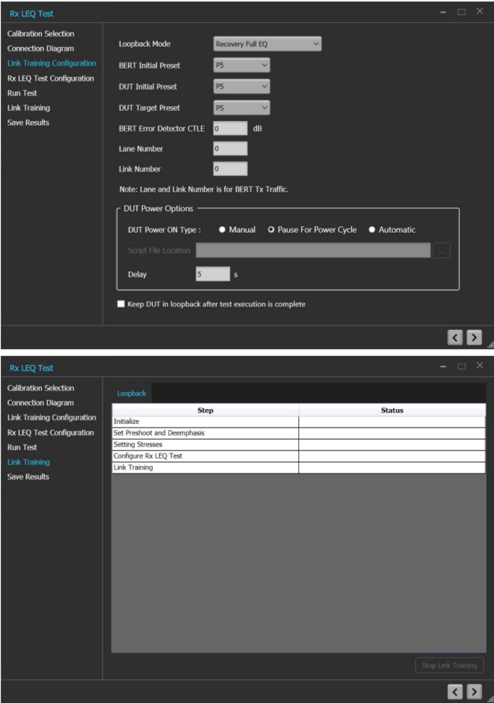
Figure 5: Flexible link training and loopback control
