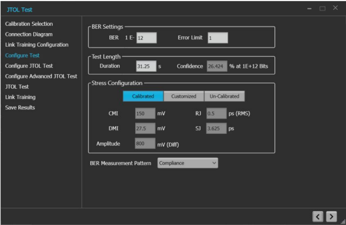
Figure 12: Error detector and stress settings for JTOL
