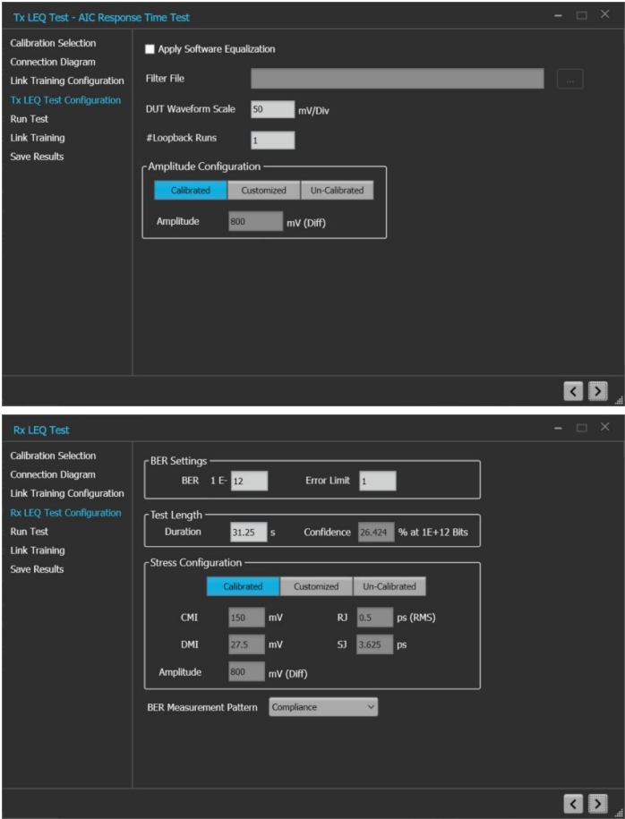
Figure 6: Tx-LEQ and Rx-LEQ test configuration
