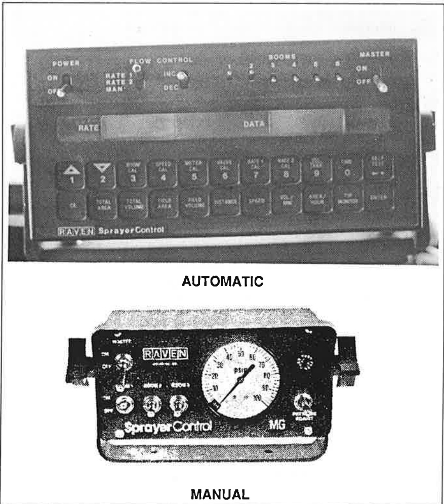
Fig. 3 SPRAY CIRCUIT CONTROLLER
