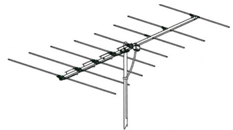
Winegard's HD6055P 10 element FM antenna (Courtesy: Winegard)
