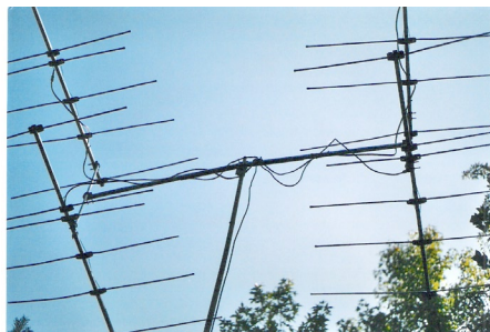
The home-brew, 24 element, stagger-stacked, quad array. First version featured an 8' long, 2 x 2 pressure treated boom that was replaced by an aluminum boom also 8' long. (Courtesy: Author)
