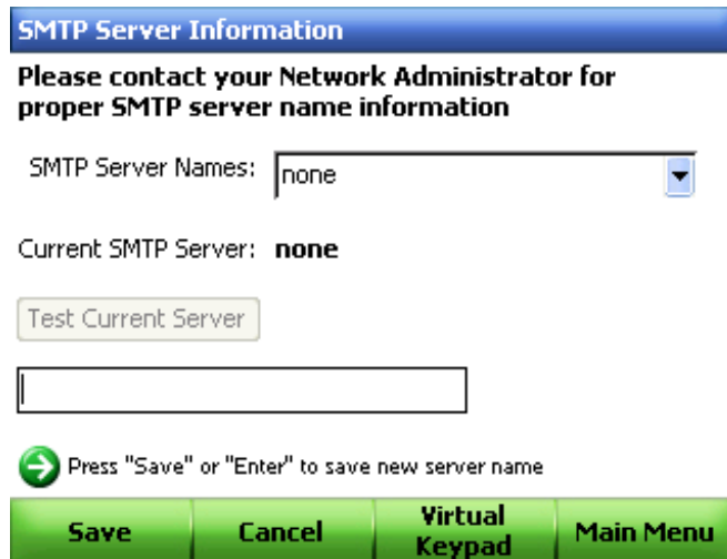
Figure 25. SMTP server setup.
