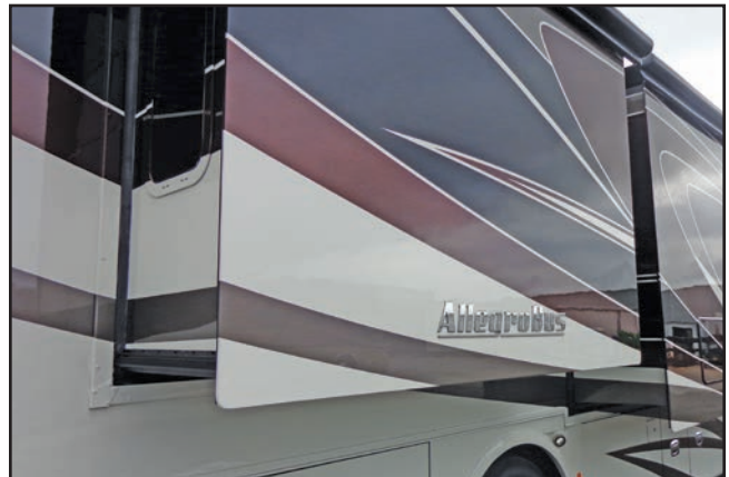
Figure 9-2: Typical slide-out fully extended
