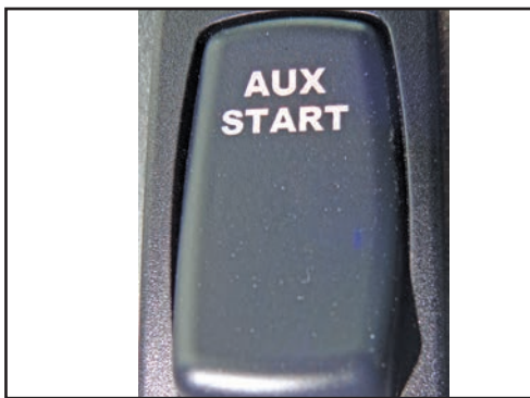
Figure 8-2: Auxiliary start switch
