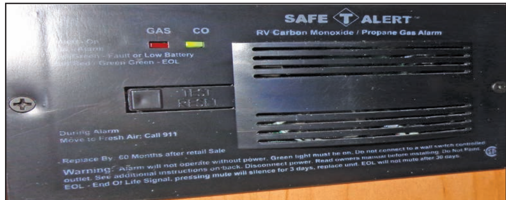
Figure 2-6: Carbon Monoxide alarm
