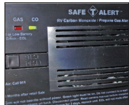
Figure 2-5: Carbon Monoxide alarm
