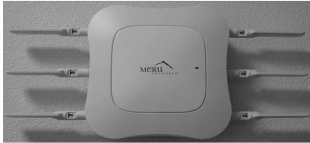
Figure 14: Horizontal Antenna Orientation (Side View)
