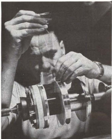
SUPERCONDUCTING magnet being wound at Westinghouse Electric
