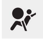
SRS warning light
